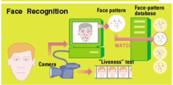
**Face-recognition** software uses a camera attached to your PC to capture and map key identifying features. Some also perform a "liveness" test to see how your face moves, so that a photo of you cannot be used.
